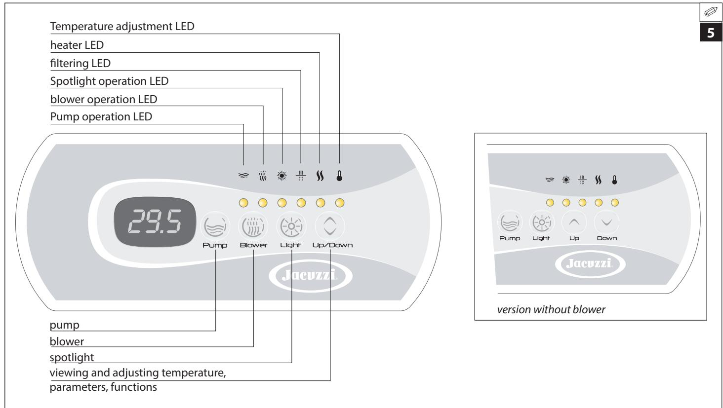
► As soon as the water temperature set point is reached, the heater is shut off. It will not be turned back on until the water temperature drops about 0.5 °C (1 °F) below the set point.
