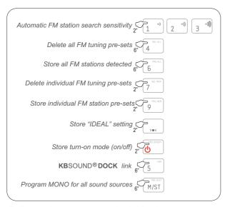
To illustrate that an operation requires holding down a key on the remote control for a specific amount of time, the symbol will appear in the manual next to the key. The screen will display the symbol.
